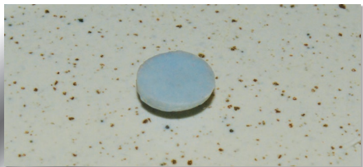
A sample of «Belabond» - ortho at a temperature 25°C (Room temperature)
